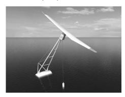
Dutch company Touchwind has an interesting spin on the idea... waka waka. It's designed around a massive single-piece rotor, sitting on the end of a pole that's draped over a big barrel, with a large floating buoy hanging beneath it.
