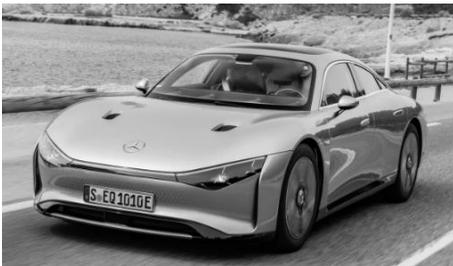
The idea was to test the vehicle in real-world conditions, and high-speed driving featured early on in the journey as the Vision EQXX took to Autobahn 81 at up to 140 km/h (87 mph) on the way to Switzerland – making the most of the concept's low drag coefficient of 0.17, achieved thanks to the flowing body shape, compact front end, specially developed Bridgestone tires with low rolling resistance and active rear diffuser that automatically deploys at speeds above 60 km/h.
