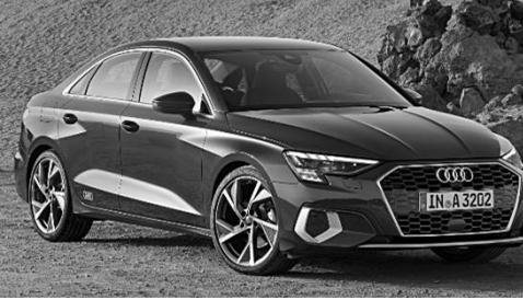
AUDI's A3 entry-level luxury sedan and its higher-performance S3 companion are redesigned for 2022. There are crisp new exterior details, and the interior looks as nice as ever. Under the hood of the 2022 Audi A3, there's a 201-horsepower, 2.0-liter 4-cylinder engine equipped with a 48-volt mild-hybrid system. The sporty S3 has a 306-hp turbo 4-cylinder. Both sedans use a 7-speed dual-clutch automatic transmission (DCT). Later in 2022, Audi will launch a new 401-hp RS 3 sedan.
