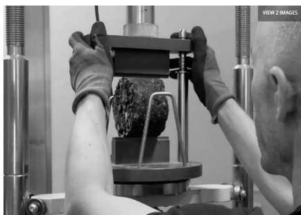
A piece of cigarette-butt-enhanced asphalt gets strength-tested.
